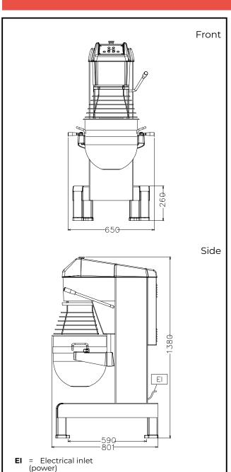
Electric Supply voltage: 600175 (DMBE40B) 200-240 V/1N ph/50/60 Hz 600176 (DMBE40B3) 380-480 V/3 ph/50/60 Hz Capacity: ISO 9001; ISO 14001 kg/ Performance (up to): Cycle 40 litres Capacity: Key Information: External dimensions, 655 mm Width: External dimensions, Depth: 850 mm External dimensions, 1370 mm Height: **Shipping weight:** 203 kg ISO 9001; ISO 14001 kg **Cold water paste:** with Spiral hook 70 with Whisk Egg whites:
